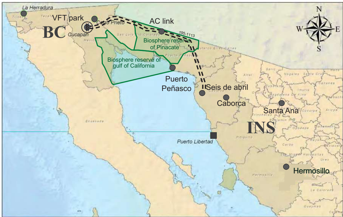
Figure 4.12: Mexican interconnection link between INS-CFE and BC-CFE systems based on VFT park.
