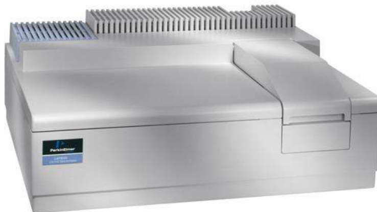
Figura 3.4 Lambda 25 UV/Visible Spectrophotometer.
