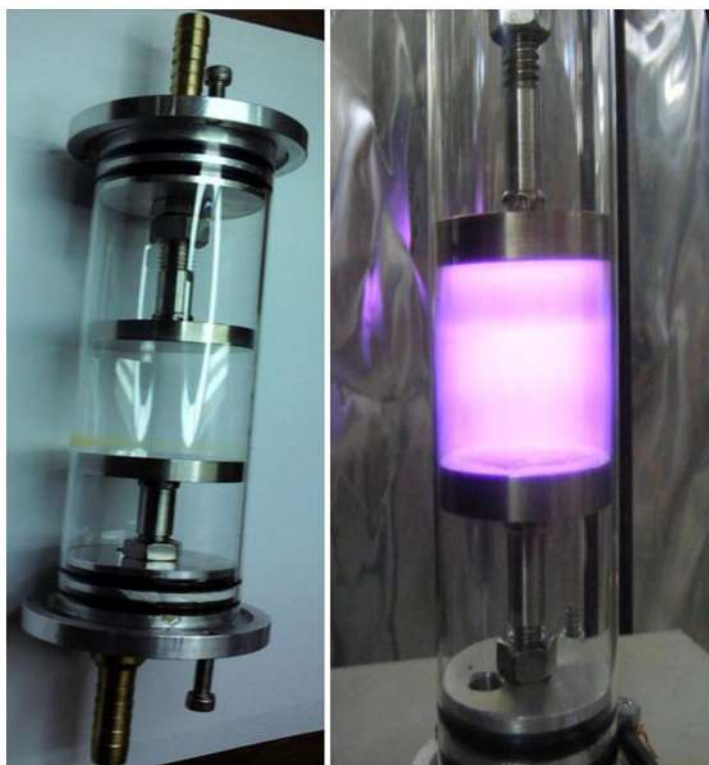
Fig. 1 Experimental set up to produce the nitrogen plasma
