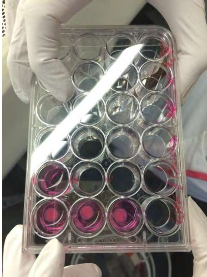
Fig. 25 Photograph of well plates containing hydrogels submerged in Cell-Culture Media for hMCS growth.
