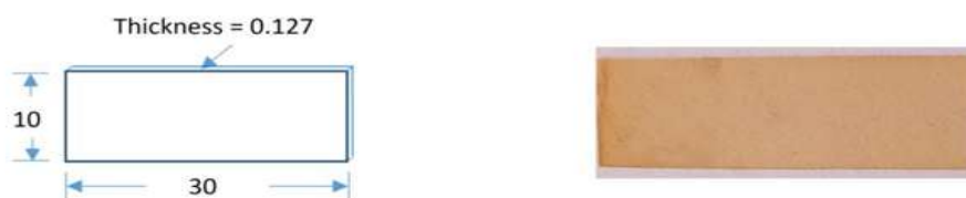
Figure 1: Dimensions (mm) of the experimental Nafion 115 strip and picture.
