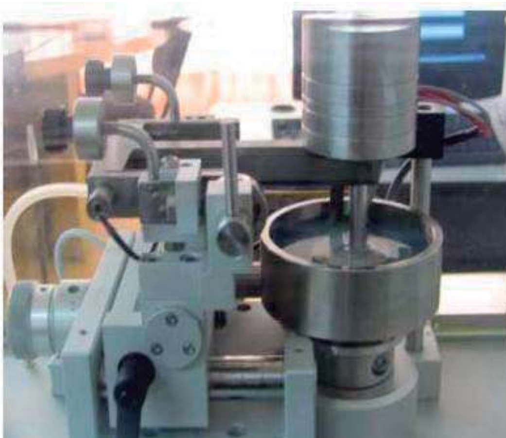
Figuras 3.5. Tribómetro Bola-Disco (ball on disk, marca Micro Photonics)
