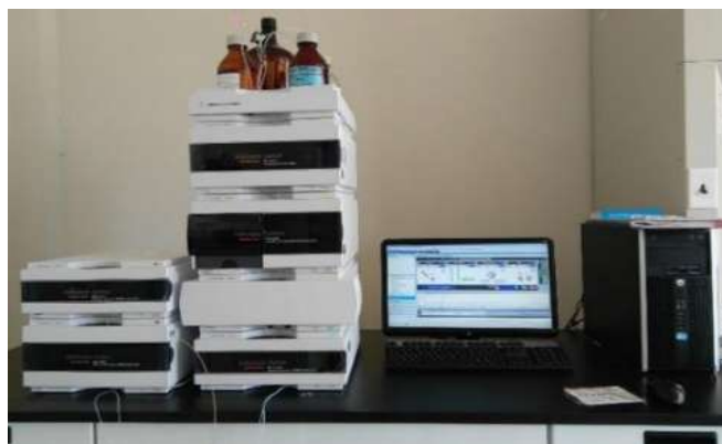
Figura 18. HPLC Agilent Technologies 1200 Infinity Series.
